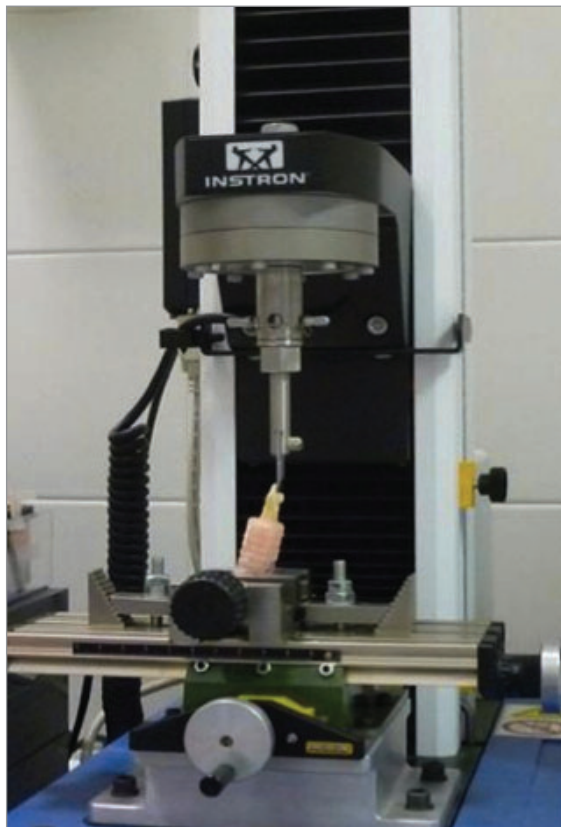
Figure 1. Universal testing machine Model 3343, Instron (Universal testing machine, Model 3343, Instron Corporation, Norwood, MA, USA).
