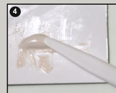
4 Spatulate thoroughly to get a homogenous void free mix
