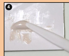
Spatulate thoroughly to get a homogenous void free mix
